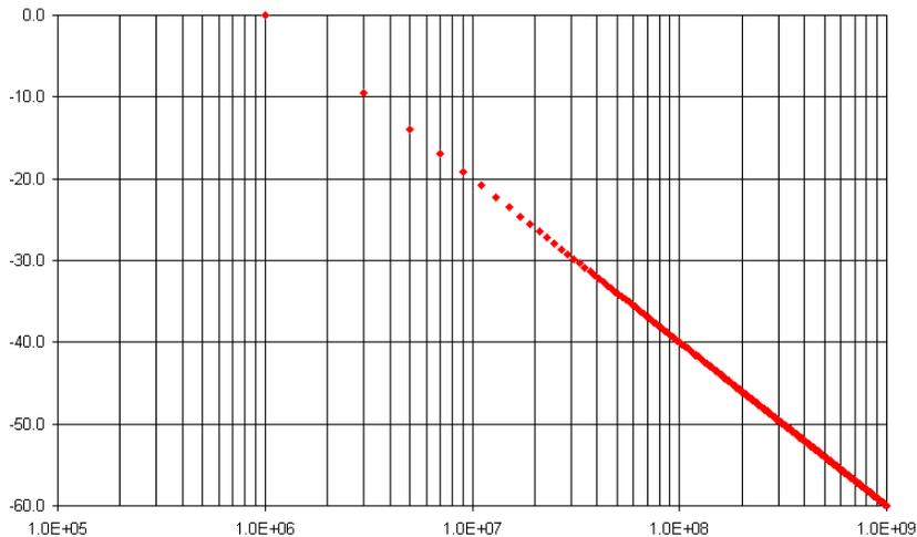
**Figure 1. The Spectrum of a 1-MHz Square Wave**
