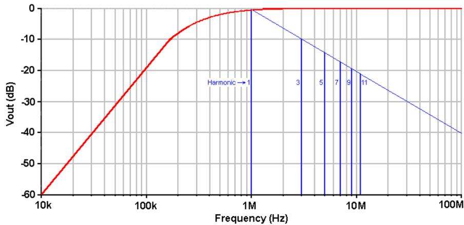
Figure 7. High Pass Filtering a Square Wave
