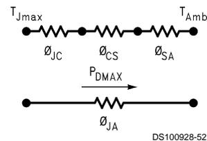
Once the maximum package power dissipation has been calculated using Equation (1), the maximum thermal resistance,  $\theta_{SA}$ , (heat sink to ambient) in  $^{\circ}\text{C}/\text{W}$  for a heat sink can be calculated. This calculation is made using Equation (3) which is derived by solving for  $\theta_{SA}$  in Equation (2).
